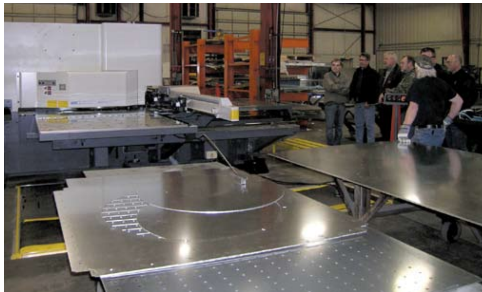
The Murata press is 100 per cent electrically operated and uses about 70 per cent less energy than other turrets, says Jonathan Barrick, marketing manager for Global Finishing's Canadian sales and design engineering arm in Barrie, ON.
