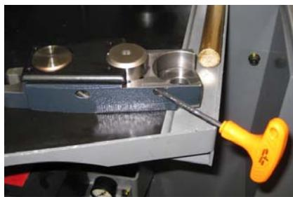
Now, with the die holder in place, keep your hand on the die holder cap holding it down, and using your torque wrench, turn it clockwise one full click. This is all that is required to securely lock the die holder in place. As a reference, your wrench should be calibrated to  $90 \pm 5$  (kgf cm).
