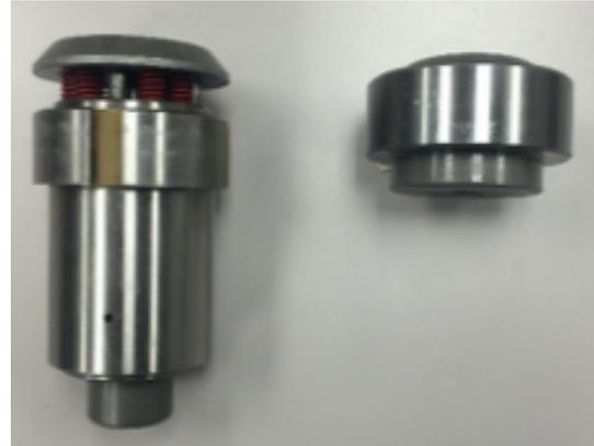
Figure 1: Retractable die (L); traditional die (R).
