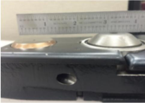
**Figure 4: Different heights with traditional forming tooling.**
